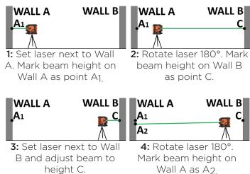
**5:** Measure the vertical distance between  $A_1$  and  $A_2$ . If this distance is smaller than 1/8" at 20', your horizontal accuracy is within specification.
